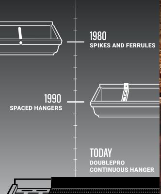
The continuous hanger is the only fastening system that leaves gutters strong and rigid along their entire length. It eliminates the weaknesses that other systems generate between nails and spaced hangers.
