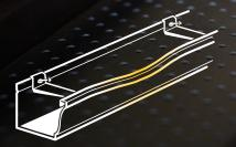
Rain gutters are commonly installed with spaced hangers that cause weak spots on the gutter between each hanger.
