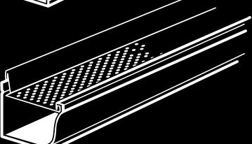
With a **continuous hanger™**, the rain gutters are reinforced along their entire length.
