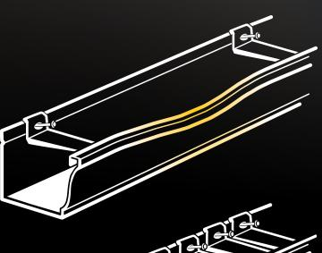
Rain gutters are commonly installed with spaced hangers that cause weak spots on the gutter between each hanger.
