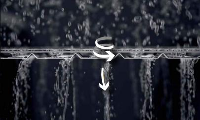
The offset holes of the **eclipse** TECHNOLOGY make it the perfect filter, allowing water to drain freely while blocking pine needles and leaves without ever getting clogged.
