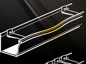
Rain gutters are commonly installed with spaced hangers that cause weak spots on the gutter between each hanger.
